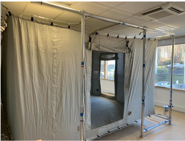
Fig.2. Picture of the experimental setup installed in the VIRC of CISTEME
