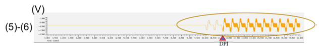
Fig.14. Signal waveforms during DPI on TPL communication bus with new transformer model.
